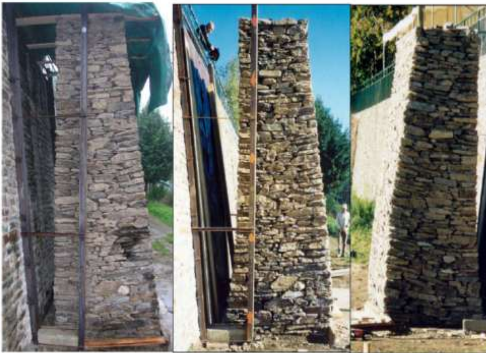
Fig. 7. Wall 5, left: before loading, centre and right: after loading "belly shape".
